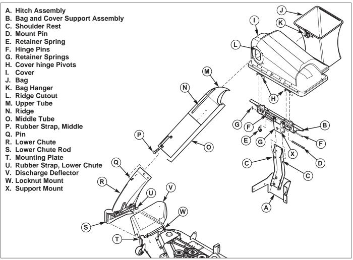
Figure 11. Normal Installation & Removal
